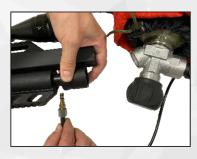
Close the valve of the pressure bottle and pull out the filling nipple.
