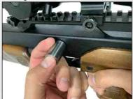
Get the magazine into position by pushing on its block from above and than from the side.
