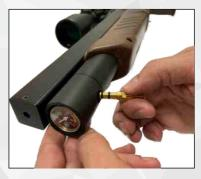
Close the valve of the pressure bottle and pull out the filling nipple.
