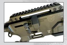
When the bolt is re-cocked, the bullet will automatically stand in front of the chamber and when the bolt is closed it will reach to put the bullet in the barrel. To keep the barrel free of bullet when re-cocking, remove the magazine from the rifle.
