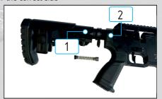
Insert the spring assembly (1) into the bolt house (2).
